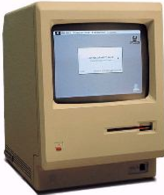
The first Macintosh computer, introduced in 1984, upgraded to a 512K "Fat Mac"
