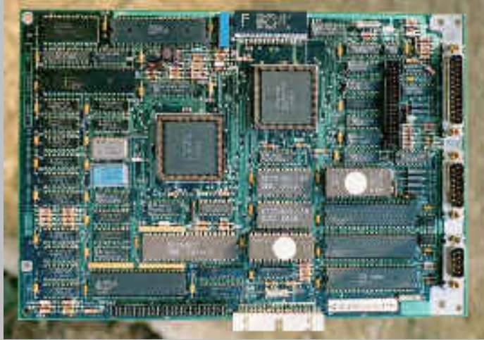
DECmate III - The Main Circuit Board.
