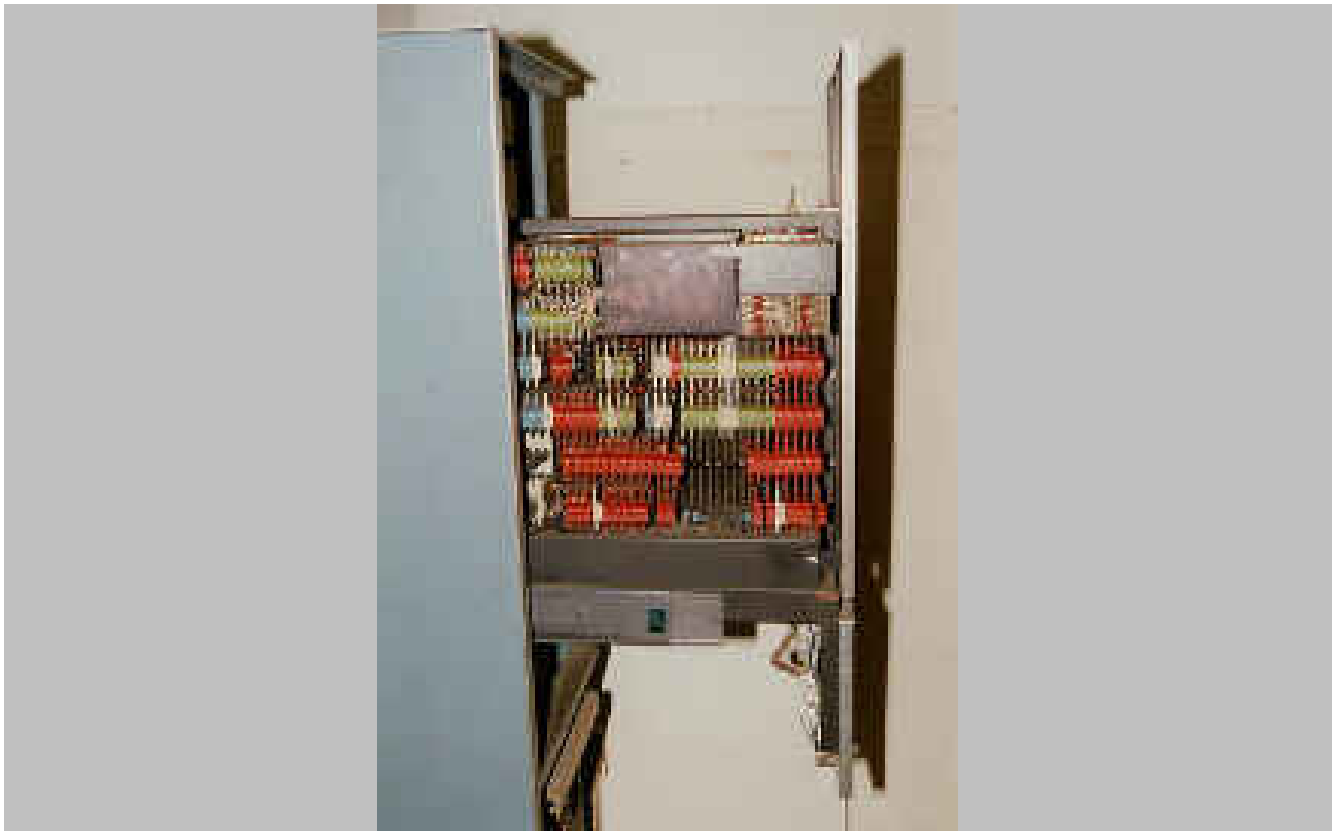
PDP-8 The Processor Side
