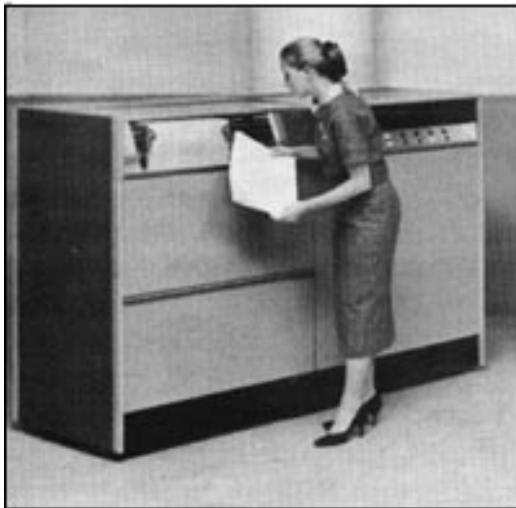
Univac Solid State High-Speed printer is capable of printing up to 600 lines per minute
