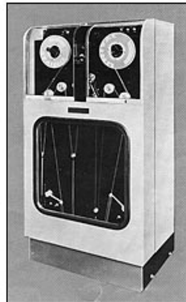
Universe III reads data at the rate of 200,000 digits per second.
