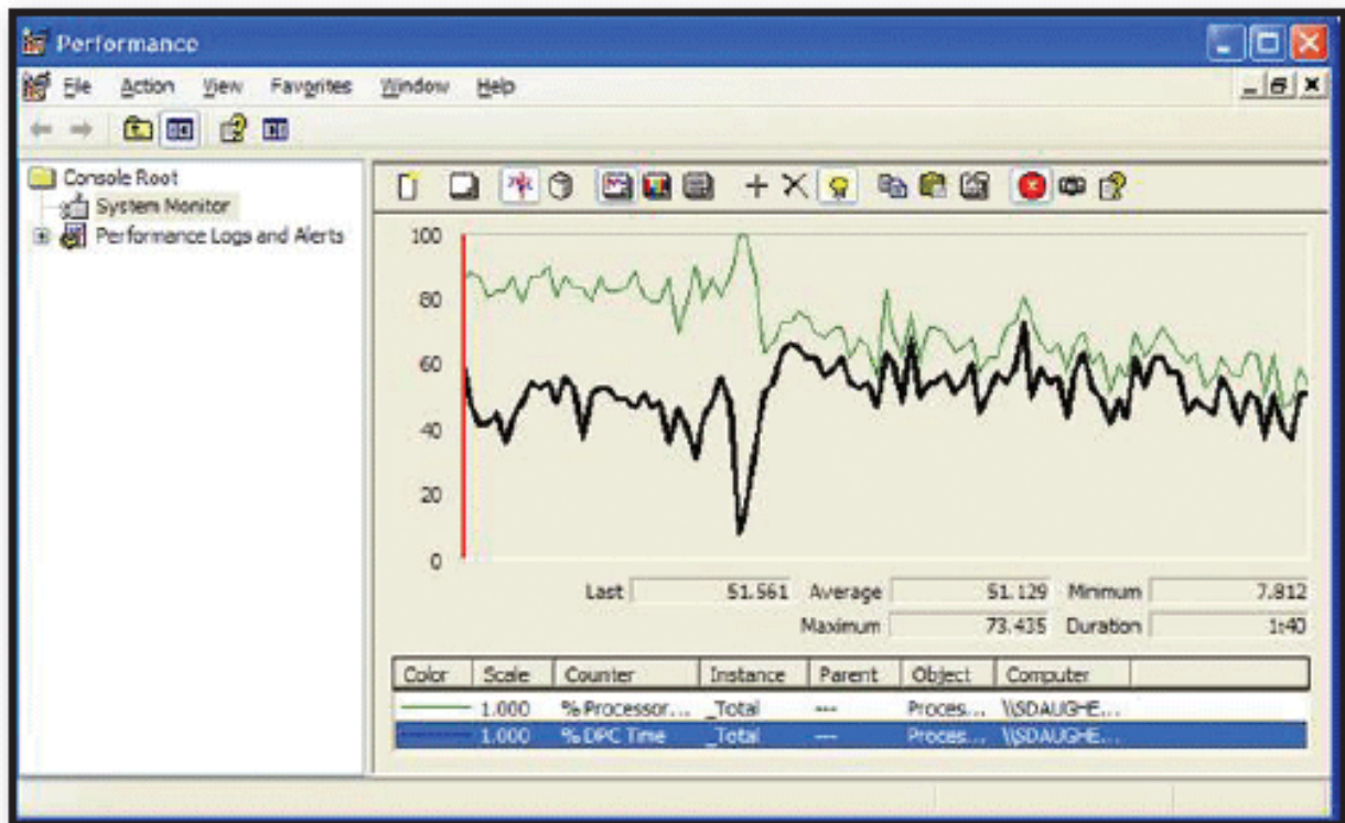
Figure 3: Using Performance Monitor to determine how much time the processor is spending on DPCs
