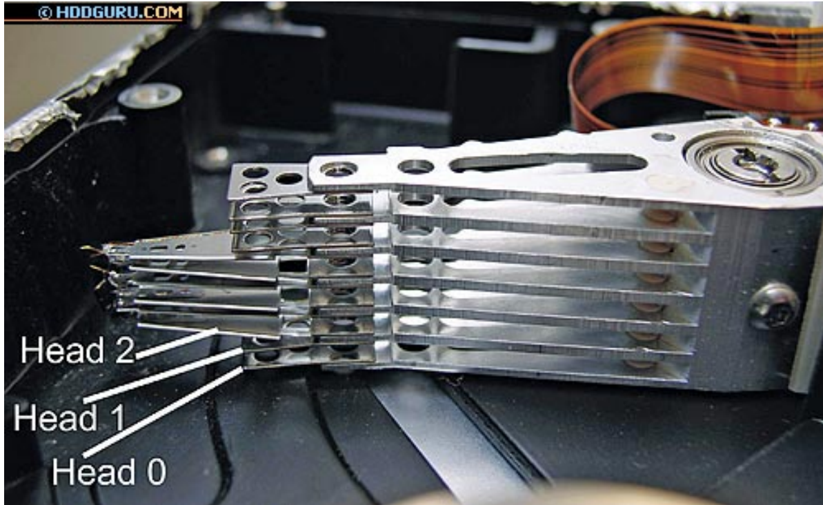
Figure 21 A heads numbering scheme (SCSI Western Digital)
