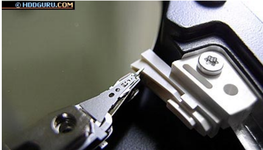
Figure 13 Heads are loaded onto the surface (Hitachi AVV2 series hard drive, 80 GB)
