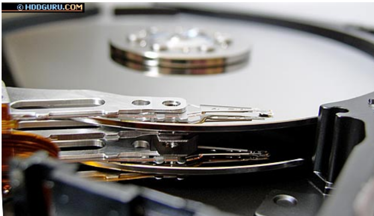
Figure 22 A head stack (WD600BB) — heads number 0, 1 and 3 are physically present; head number 2 is missed
