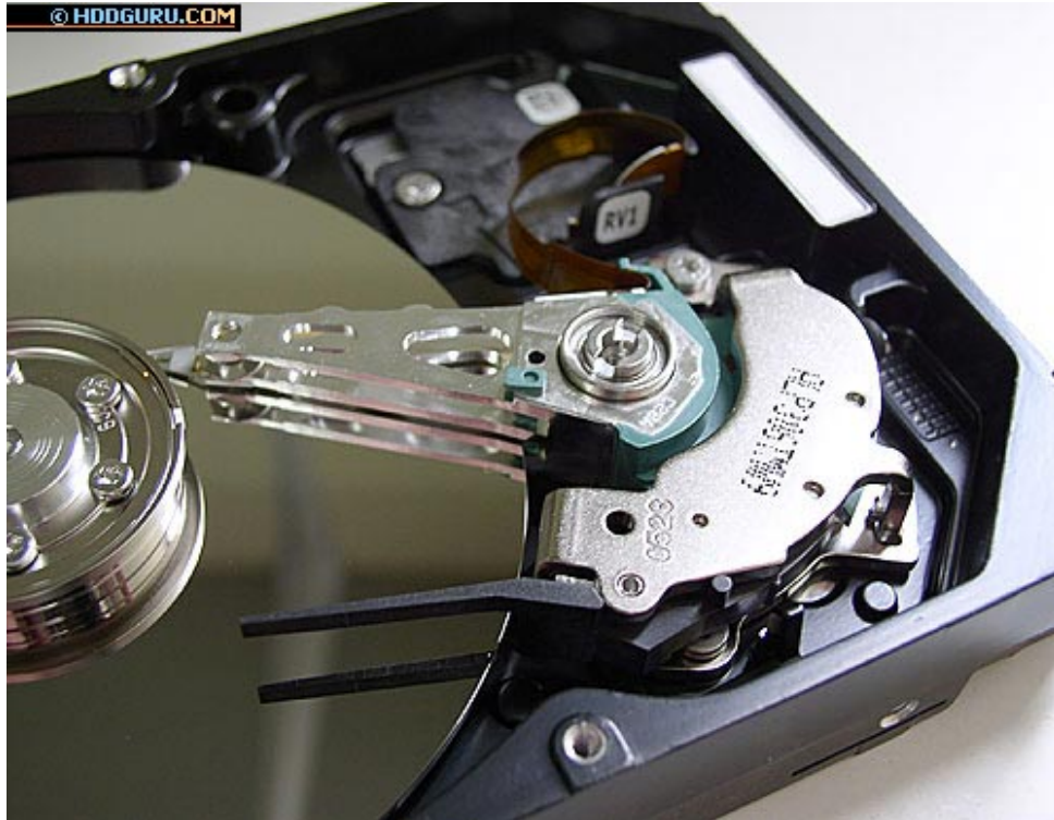
Figure 9 The same drive with a plastic airlock visible
