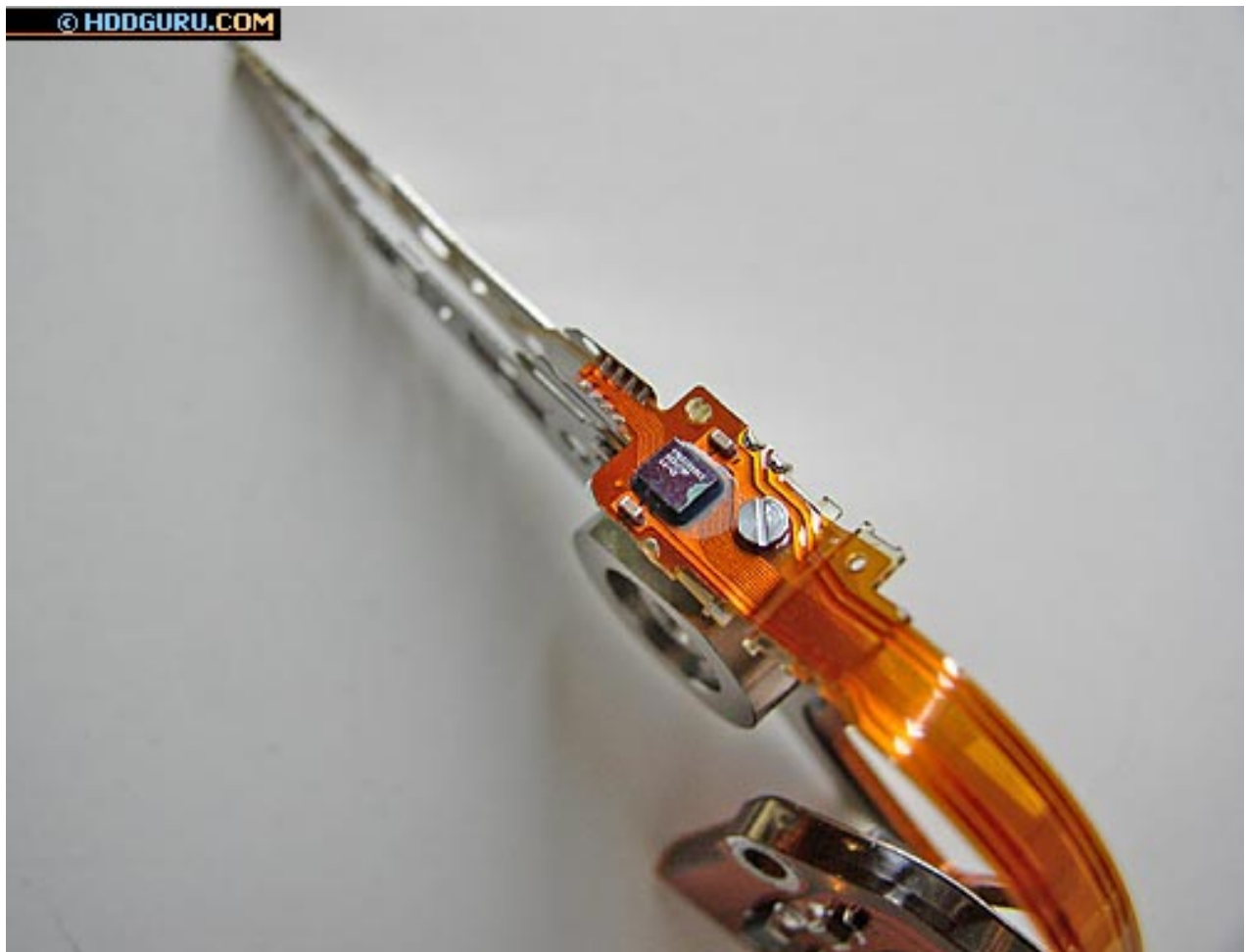
Figure 1 A head stack with an open-frame preamplifier (Hitachi ATMR series, 2.5-inch drive)
