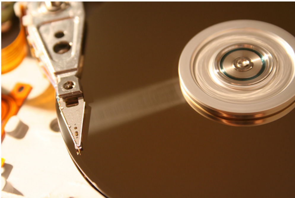
Figure 1.2: A hard disk spinning while the head accesses the data (Source: http://www.flickr.com/photos/alphasix/179676660 ).
