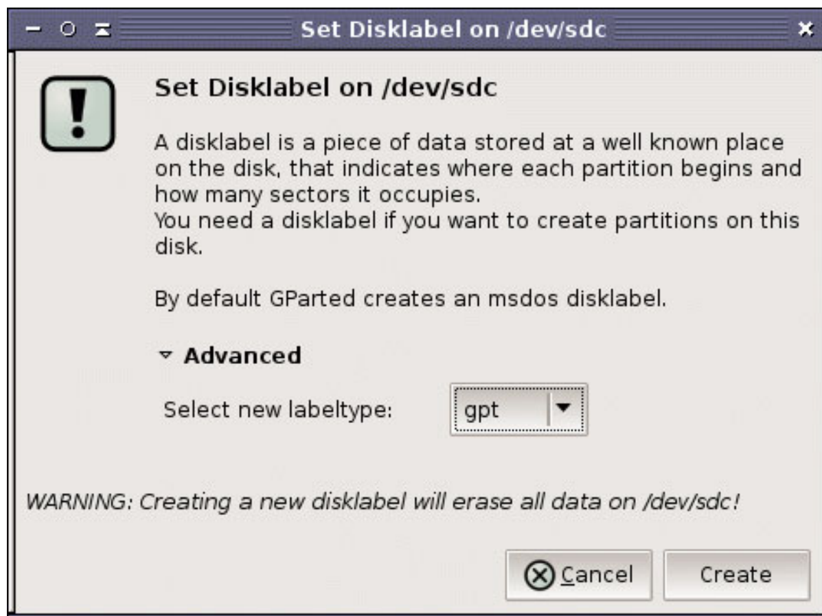
Figure 2. You must explicitly set the GPT label type to create GPT partitions in the GNOME Partition Editor
