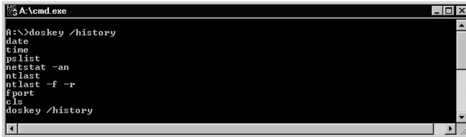
Figure 13: Using doskey to record the steps taken during incident response
