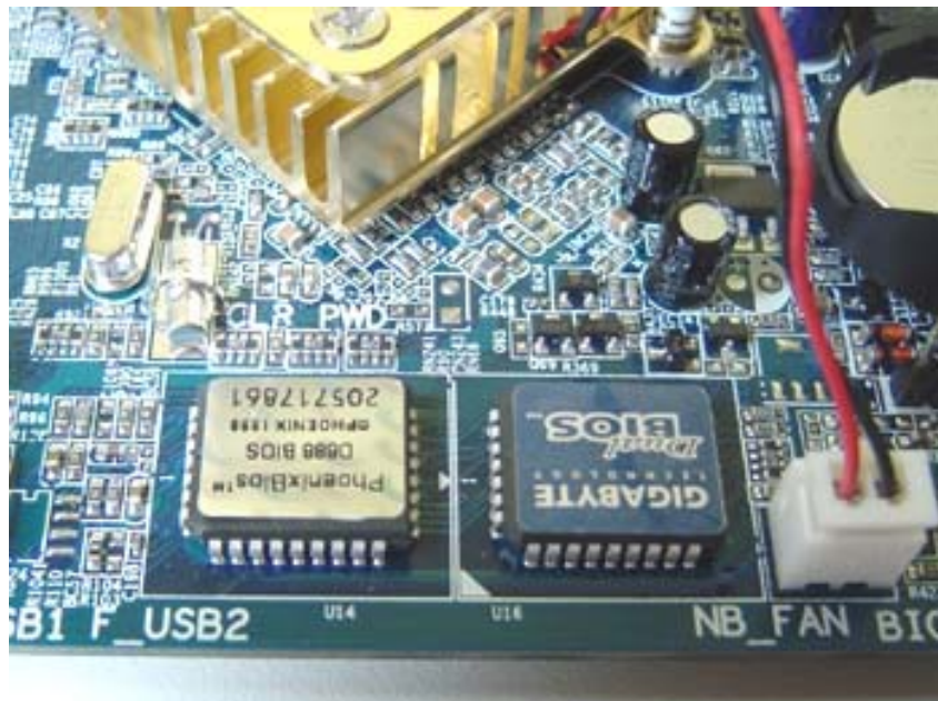
Figure 2: Detail of a motherboard from Gigabyte with the Dual BIOS feature
