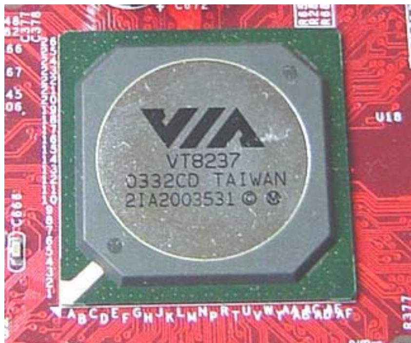
Figure 2 Example of a south bridge chip. The CMOS memory and the Real Time Clock (RTC) are both embedded in this chip nowadays.
