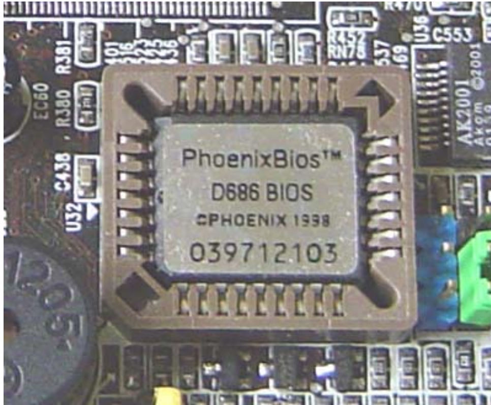
Figure 1 Motherboard ROM memory chip. BIOS, POST and Setup softwares are written in this chip.
