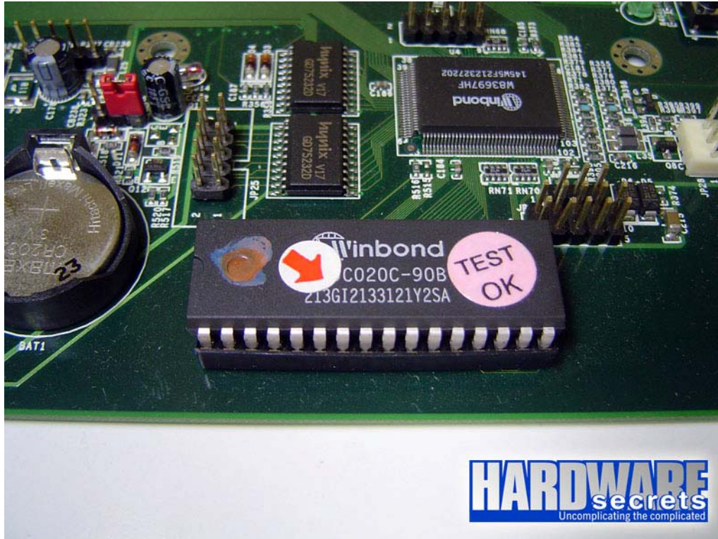
Figure 1: The BIOS chip. This kind of chip is called DIP (Dual In-Line Package)
