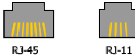
Figure: Diagram of Ethernet (RJ-45) socket compared with telephone (RJ-11) jack. RJ45 has 8 wires, RJ11 has 2 or 4.
