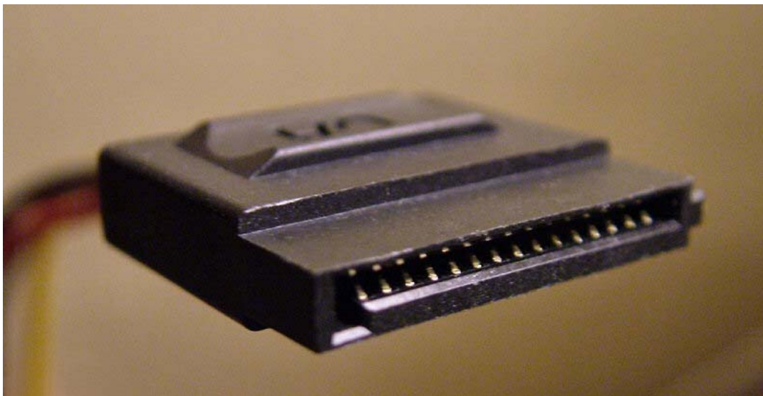
A 15-pin Serial ATA power receptacle. This connector does not provide the extended pins 4 and 12 needed for hot-plugging.
