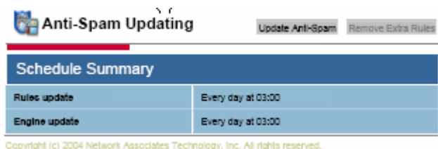
Figure 3.10: The automatic update facility allows for separate scheduling of signature file (rules) and scanner (engine) updates.
