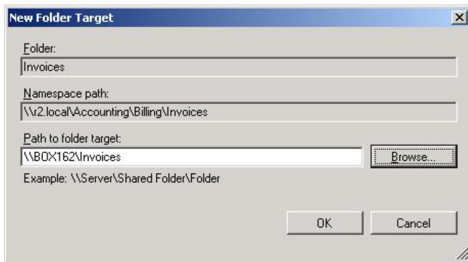
Figure 3 Adding a second folder target for the Invoices folder in the \\r2.local\Accounting namespace
