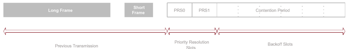
Figure 3: Priority Resolution and Backoff scheme
