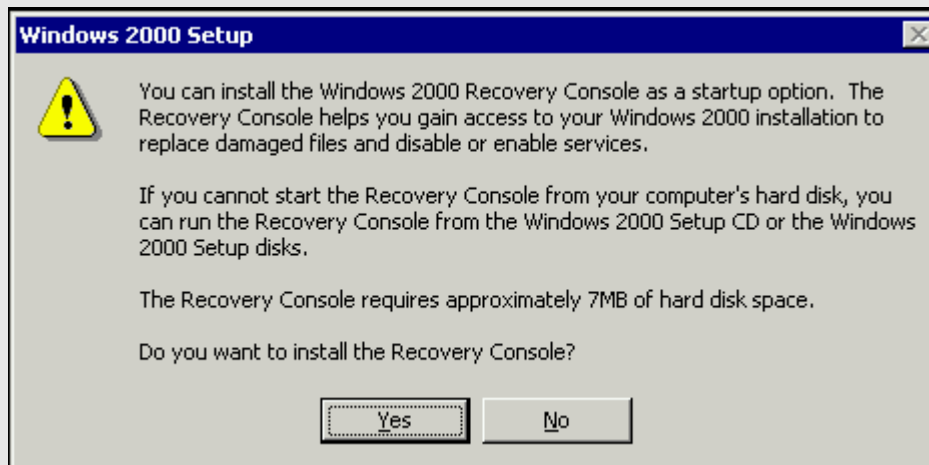
Figure 8.3: Installing the Recovery Console.
