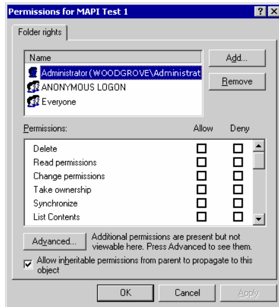
Figure 3.6 Windows 2000 Permissions dialog box for a folder in the default Public Folders hierarchy
