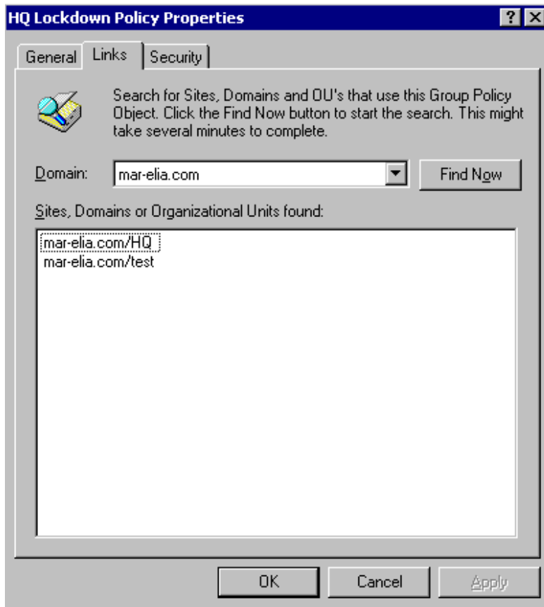
Figure 6.4: Using the Group Policy MMC snap-in's Link Search feature to find all of the links to a GPO.
