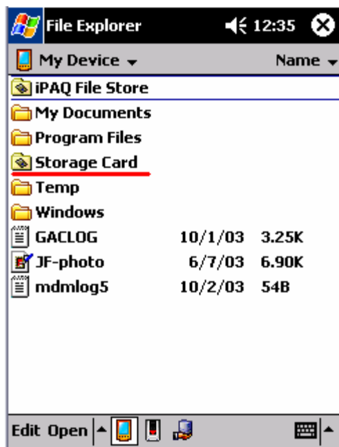
Figure 3.4: The card appears to the end user as a directory folder in the device's file system.
